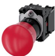
EMERGENCY STOP mushroom pushbutton, 22 mm, round, plastic, red, 40 mm, positive latching, acc. to EN ISO 13850, rotate-to-unlatch, without yellow backing plate, with holder, 1 NC, 1 NC, screw terminal
