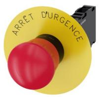
EMERGENCY STOP mushroom pushbutton, 22 mm, round, plastic, red, 40 mm, positive latching, acc. to EN ISO 13850, rotate-to-unlatch, with yellow backing plate, inscription: Arrêt d'urgence, with holder, 1 NO+1 NC, screw terminal
