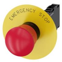
EMERGENCY STOP mushroom pushbutton, 22 mm, round, plastic, red, 40 mm, positive latching, acc. to EN ISO 13850, rotate-to-unlatch, with yellow backing plate, inscription: EMERGENCY STOP, with holder, 1 NO+1 NC, screw terminal
