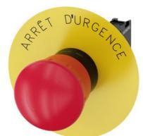
EMERGENCY STOP mushroom pushbutton, 22 mm, round, plastic, red, 40 mm, positive latching, acc. to EN ISO 13850, rotate-to-unlatch, with yellow backing plate, inscription: Arrêt d'urgence, with holder, 1 NC, screw terminal
