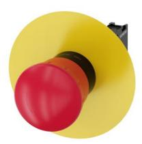
EMERGENCY STOP mushroom pushbutton, 22 mm, round, plastic, red, 40 mm, positive latching, acc. to EN ISO 13850, rotate-to-unlatch, with yellow backing plate, without inscription, with holder, 1 NC, screw terminal
