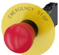
EMERGENCY STOP mushroom-type actuator, 22 mm, round, plastic, red, 40 mm, positive latching, according to EN ISO 13850, pull-to-unlatch mechanism, with yellow backing plate, inscription: EMERGENCY STOP, with holder, 1 NO+1 NC, screw terminal
