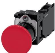
Mushroom pushbutton, 22 mm, round, plastic, red, 40 mm, latching, pull-to-unlatch mechanism, with holder, 1 NO+1 NC, Spring-type terminal
