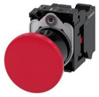
Mushroom pushbutton, 22 mm, round, plastic, red, 40 mm, latching, pull-to-unlatch mechanism, with holder, 1 NC, Spring-type terminal
