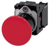
Mushroom pushbutton, 22 mm, round, plastic, red, 40 mm, latching, pull-to-unlatch mechanism, with holder, 1 NC, screw terminal
