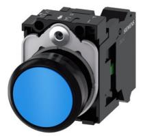
Pushbutton, 22 mm, round, plastic, blue, pushbutton, flat, momentary contact type, with holder 1 NO, Spring-type terminal  $\,$
