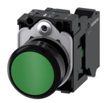
Pushbutton, 22 mm, round, plastic, green, pushbutton, flat, momentary contact type, with holder 1 NO, Spring-type terminal  $\,$
