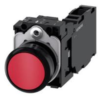
Pushbutton, 22 mm, round, plastic, red, pushbutton, flat, momentary contact type, with holder 1 NO+1 NC, screw terminal,
