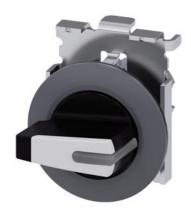
Selector switch, illuminable, 30 mm, round, metal, matte, white, knob, short, front ring for flush installation, 3 switch positions I>O<II, momentary contact type, actuating angle  $2x45^{\circ}$ , 13:30h/15h/16:30h
