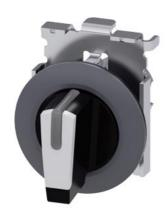
Selector switch, illuminable, 30 mm, round, metal, matte, white, selector switch, short, front ring for flush installation, 3 switch positions I>O<II, momentary contact type, actuating angle  $2x45^{\circ}$ , 10:30h/12h/13:30h
