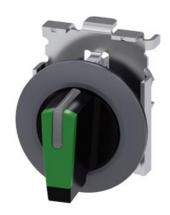
Selector switch, illuminable, 30 mm, round, metal, matte, green, selector switch, short, front ring for flush installation, 3 switch positions I>O<II, momentary contact type, actuating angle  $2x45^{\circ}$ , 10:30h/12h/13:30h
