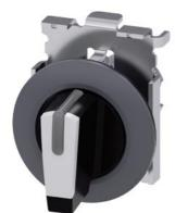
Selector switch, illuminable, 30 mm, round, metal, matte, white, selector switch, short, front ring for flush installation, 3 switch positions I-O-II, latching, actuating angle  $2x45^{\circ}$ , 10:30h/12h/13:30h
