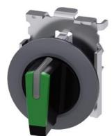
Selector switch, illuminable, 30 mm, round, metal, matte, green, selector switch, short, front ring for flush installation, 3 switch positions I-O-II, latching, actuating angle  $2x45^{\circ}$ , 10:30h/12h/13:30h
