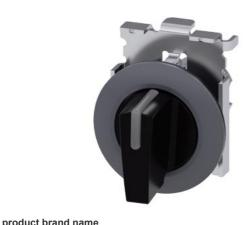
Illuminable selector switch, 30 mm, round, Metal matte, black, Selector switch short, front ring for flush installation, latching, actuating angle  $2x45^\circ$ , 10:30h/12h/13:30h
