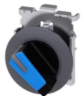
llluminable selector switch, 30 mm, round, Metal matte, blue, Selector switch short, front ring for flush installation, 2 switch positions O-I, latching, actuating angle  $90^{\circ}$ , 10:30h/13:30h
