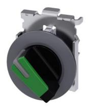
Selector switch, illuminable, 30 mm, round, metal, matte, green, selector switch, short, front ring for flush installation, 2 switch positions O-I, latching, actuating angle  $90^\circ$ , 10:30h/13:30h
