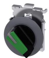
Selector switch, illuminable, 30 mm, round, metal, matte, green, selector switch, short, front ring for flush installation, 2 switch positions O<1, momentary contact type, Actuating angle 45°, 10:30h/12h
