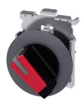
Selector switch, illuminable, 30 mm, round, metal, matte, red, selector switch, short, front ring for flush installation, 2 switch positions O<I, momentary contact type, Actuating angle  $45^\circ,\,10:30h/12h$
