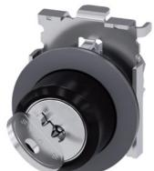
RONIS key-operated switch, 30 mm, round, metal, matte, front ring for flush installation, lock number SB30, with 2 keys, 2 switch positions O-I, latching, actuating angle 90°, 10:30h/13:30h, key removal O+I, possible special locks: SB31, 421, 455
