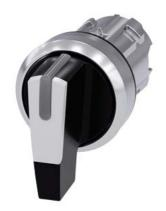
Selector switch, illuminable, 22 mm, round, metal, shiny, white, selector switch, long, 3 switch positions I>O<II, momentary contact on the left, latching on the right, actuating angle  $2x45^{\circ}$ , 10:30h/12h/13:30h
