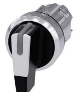
Selector switch, illuminable, 22 mm, round, metal, shiny, white, selector switch, long, 3 switch positions I-O<II, left latching, right momentary contact type, actuating angle  $2x45^{\circ}$ , 10:30h/12h/13:30h
