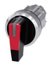
Selector switch, illuminable, 22 mm, round, metal, shiny, red, selector switch, long, 3 switch positions I-O<II, left latching, right momentary contact type, actuating angle  $2x45^{\circ}$ , 10:30h/12h/13:30h
