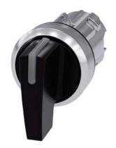
Illuminable selector switch, 22 mm, round, metal shiny, black, Selector switch long, 3 switch positions I-O<II, left latching, right momentary contact type, actuating angle  $2x45^{\circ}$ , 10:30h/12h/13:30h
