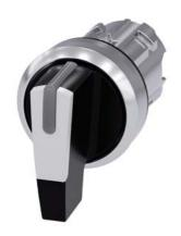
Selector switch, illuminable, 22 mm, round, metal, shiny, white, selector switch, long, 3 switch positions I>O<II, momentary contact type, actuating angle 2x45°, 10:30h/12h/13:30h
