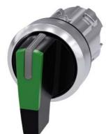
Selector switch, illuminable, 22 mm, round, metal, shiny, green, selector switch, long, 3 switch positions I>O<II, momentary contact type, actuating angle 2x45°, 10:30h/12h/13:30h
