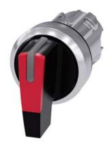
Selector switch, illuminable, 22 mm, round, metal, shiny, red, selector switch, long, 3 switch positions I>O<II, momentary contact type, actuating angle 2x45°, 10:30h/12h/13:30h
