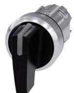
Illuminable selector switch, 22 mm, round, metal shiny, black, Selector switch long, 3 switch positions I>O<II, momentary contact type, actuating angle 2x45°, 10:30h/12h/13:30h
