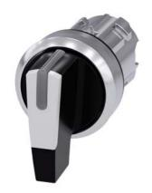
Selector switch, illuminable, 22 mm, round, metal, shiny, white, selector switch, long, 3 switch positions I-O-II, latching, actuating angle  $2x45^\circ$ , 10:30h/12h/13:30h
