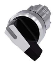
Selector switch, illuminable, 22 mm, round, metal, shiny, white, selector switch, long, 2 switch positions O-I, latching, actuating angle 90°, 10:30h/13:30h
