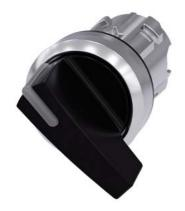
Illuminable selector switch, 22 mm, round, metal shiny, black, Selector switch long, 2 switch positions O-I, latching, actuating angle  $90^\circ$ , 10:30h/13:30h
