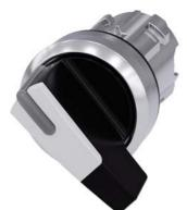
Selector switch, illuminable, 22 mm, round, metal, shiny, white, selector switch, long, 2 switch positions O<I, momentary contact type, Actuating angle 45°, 10:30h/12h
