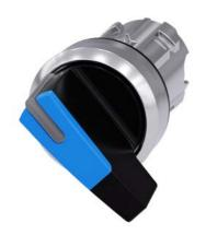
Selector switch, illuminable, 22 mm, round, metal, shiny, blue, selector switch, long, 2 switch positions O<I, momentary contact type, Actuating angle 45°, 10:30h/12h
