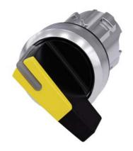
Selector switch, illuminable, 22 mm, round, metal, shiny, yellow, selector switch, long, 2 switch positions O<I, momentary contact type, Actuating angle  $45^\circ$ , 10:30h/12h
