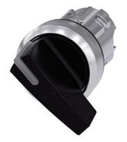
Illuminable selector switch, 22 mm, round, metal shiny, black, Selector switch long, 2 switch positions O<I, momentary contact type, Actuating angle  $45^\circ$ , 10:30h/12h
