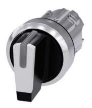
Selector switch, illuminable, 22 mm, round, metal, shiny, white, selector switch, short, 3 switch positions I>O<II, momentary contact on the left, latching on the right, actuating angle  $2x45^{\circ}$ , 10:30h/12h/13:30h
