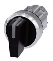
Illuminable selector switch, 22 mm, round, metal shiny, black, Selector switch short, 3 switch positions I>O<II, momentary contact on the left, latching on the right, actuating angle  $2x45^{\circ}$ , 10:30h/12h/13:30h
