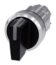
Illuminable selector switch, 22 mm, round, metal shiny, black, Selector switch short, 3 switch positions I-O<II, left latching, right momentary contact type, actuating angle  $2x45^{\circ}$ , 10:30h/12h/13:30h
