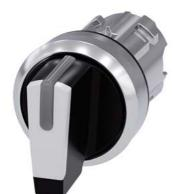
Selector switch, illuminable, 22 mm, round, metal, shiny, white, selector switch, short, 3 switch positions I>O<II, momentary contact type, actuating angle  $2x45^{\circ}$ , 10:30h/12h/13:30h
