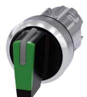
Selector switch, illuminable, 22 mm, round, metal, shiny, green, selector switch, short, 3 switch positions I>O<II, momentary contact type, actuating angle 2x45°, 10:30h/12h/13:30h
