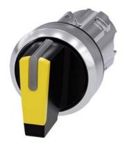
Selector switch, illuminable, 22 mm, round, metal, shiny, yellow, selector switch, short, 3 switch positions I>O<II, momentary contact type, actuating angle 2x45°, 10:30h/12h/13:30h
