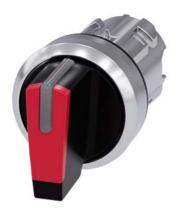
Selector switch, illuminable, 22 mm, round, metal, shiny, red, selector switch, short, 3 switch positions I>O<II, momentary contact type, actuating angle 2x45°, 10:30h/12h/13:30h
