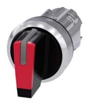
Selector switch, illuminable, 22 mm, round, metal, shiny, red, selector switch, short, 3 switch positions I-O-II, latching, actuating angle  $2x45^\circ$ , 10:30h/12h/13:30h
