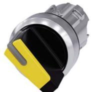
Selector switch, illuminable, 22 mm, round, metal, shiny, yellow, selector switch, short, 2 switch positions O<I, momentary contact type, Actuating angle 45°, 10:30h/12h
