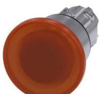
Illuminated mushroom pushbutton, 22 mm, round, metal, shiny, amber, 40 mm, latching, Pull-to-unlatch mechanism
