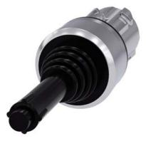
coordinate switch, 22 mm, round, metal shiny, black, 4 switch positions, momentary contact type, with mechanical interlocking  $\,$
