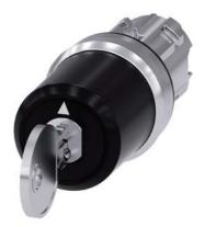
Key-operated switch BKS, 22 mm, round, metal, shiny, lock number S1, with 2 keys, 3 switch positions I-O<II, left latching, right momentary contact type, actuating angle  $2x45^{\circ}$ , 10:30h/12h/13:30h, Key removal O+I
